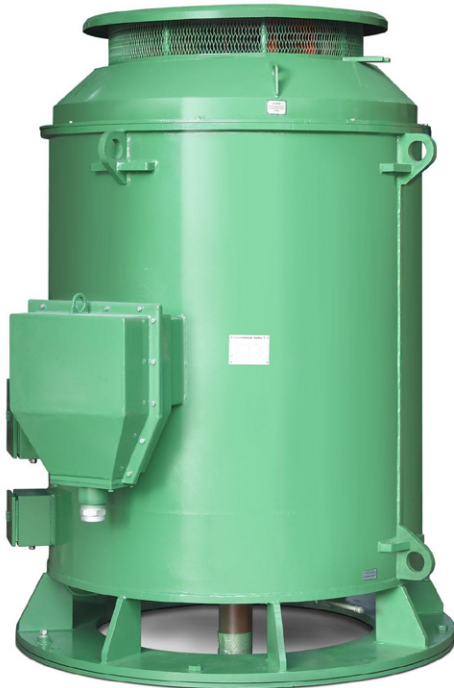
SQUIRREL CAGE MOTOR TYPE CM 630 L8 1150 kW – 5500 V – 50 Hz – 750 rpm – 8P – V1 – IP55 FOR WATER PUMP
