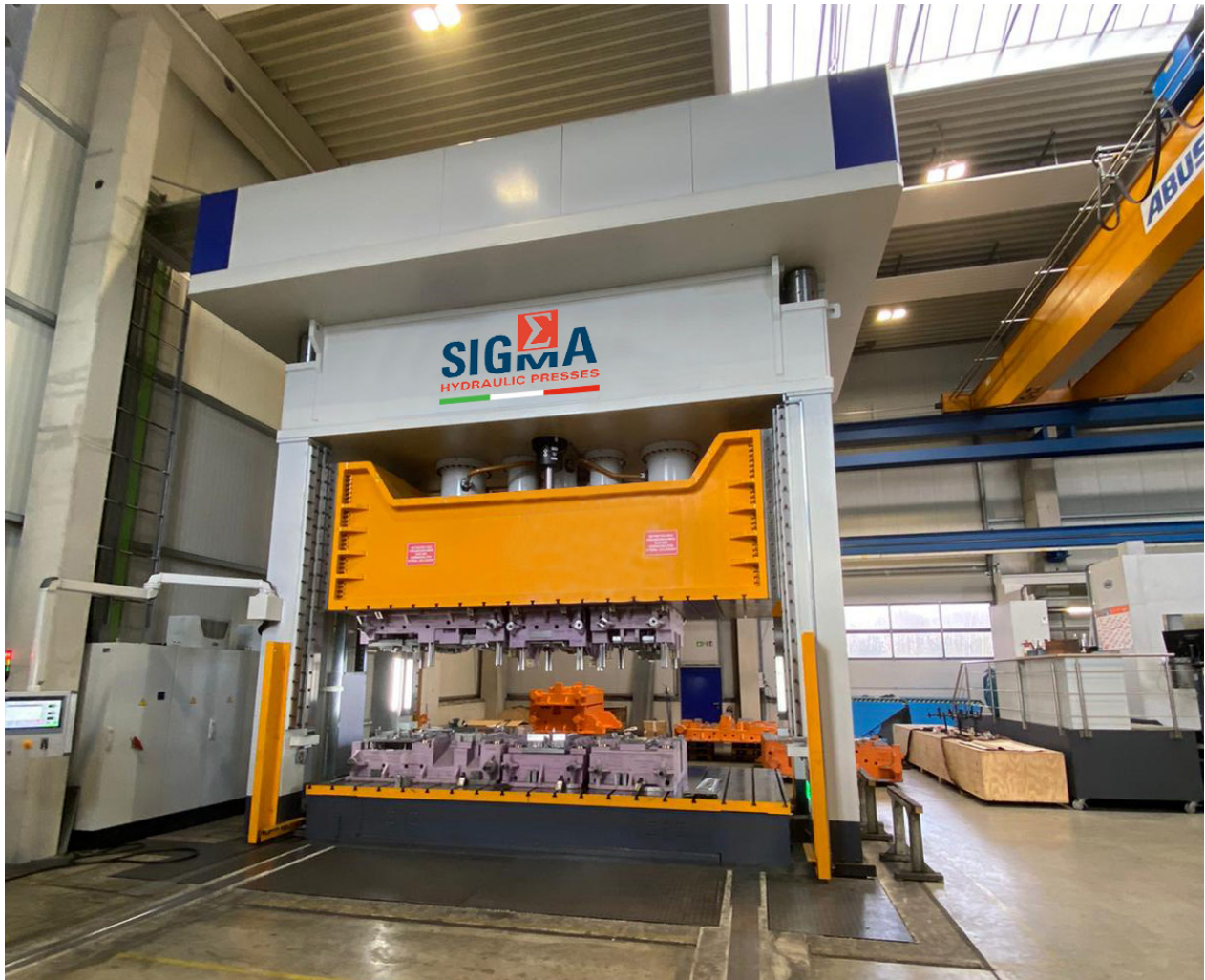
1200Ton Servo Hydraulic Press for automotive
